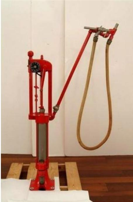
This 1916 Bowser gasoline pump operated by a hand crank and “clock face” dial. Photo from the Smithsonian Collection.
